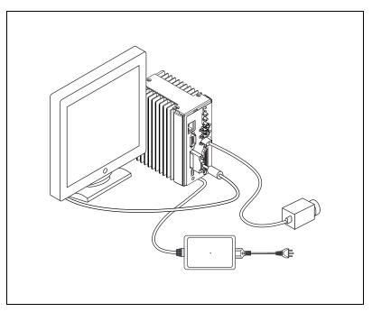
Figure 5-3. CVS-1450 Device Connected to a Monitor
